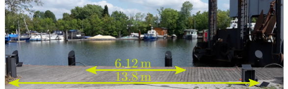
(a) Transmission distances d_{\text{LOS}} . The hydrophones were mounted with a distance of approximately 1.7 m to the jettie and at a depth of 1.1 m.
